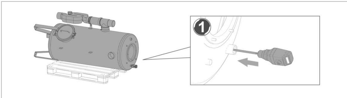
1. Insert the measuring rod of the level probe into the opening provided for this purpose.
