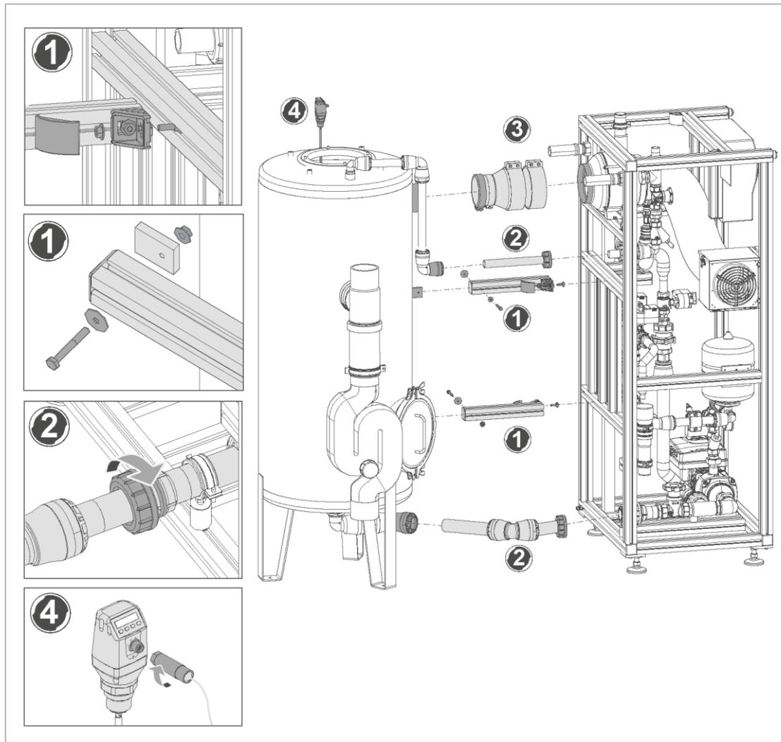
1. Screw the system rack to the filter tank.
