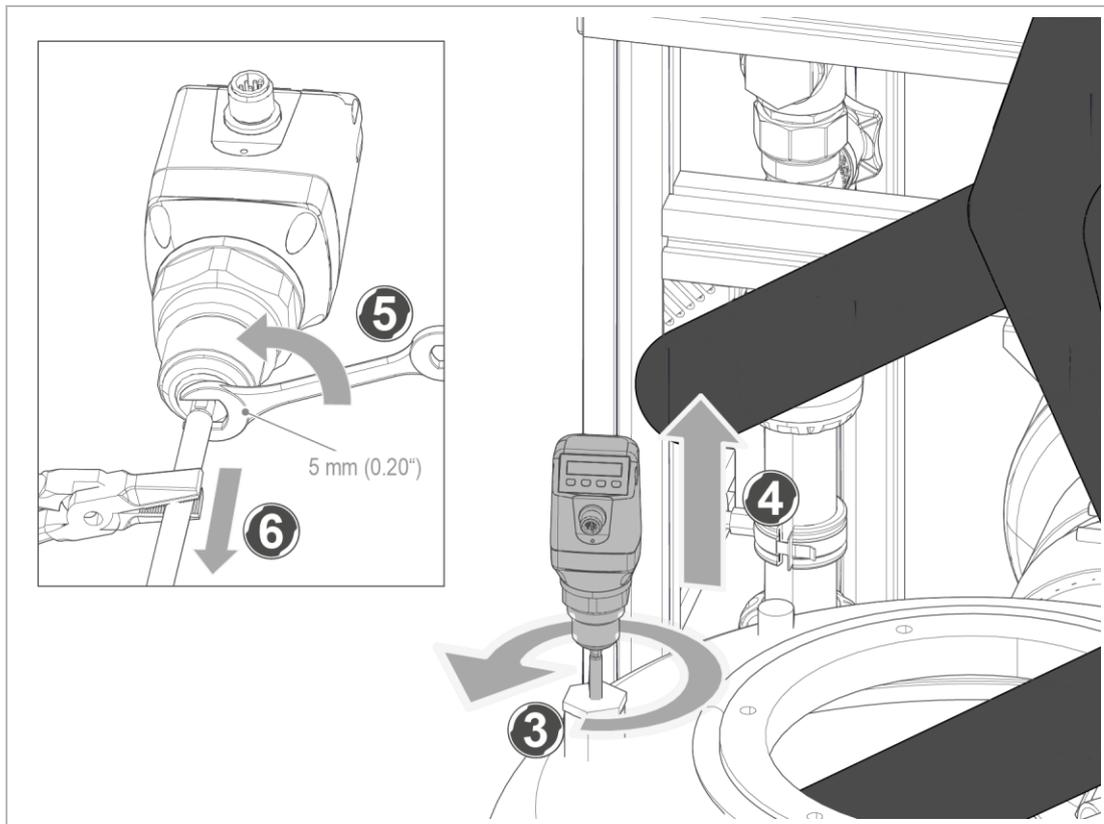
3. Unscrew the top part of the level probe from the tank.
