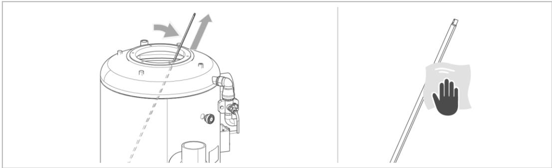
6. Grasp the rod through the opening of the tank and push it down until it can be pulled out of the tank opening by tilting it.
