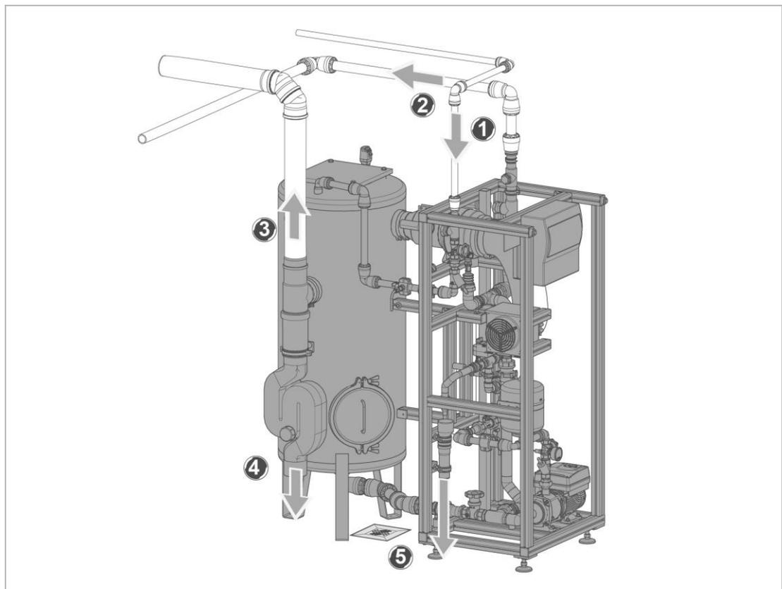
1. Connect the inlet pipe to the “raw water inlet” connection.
